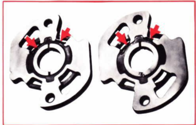
Figure 21—Damaged Upper and Lower Pressure Plates
