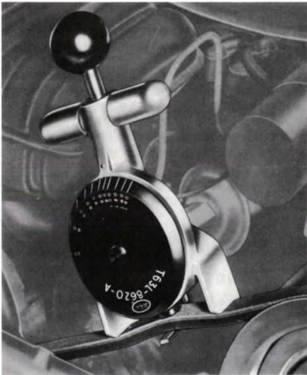
Figure 2—Checking Drive Belt Tension
