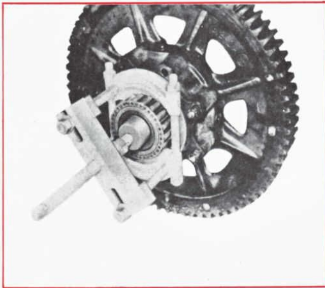
Figure 16 – Using a bearing puller. Be sure and pull in a straight line.
