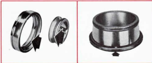
Figure 24 and 25 – Indented and scarred raceways from metal particles.
