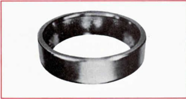
Figure 23 – Typical abrasive wear.
