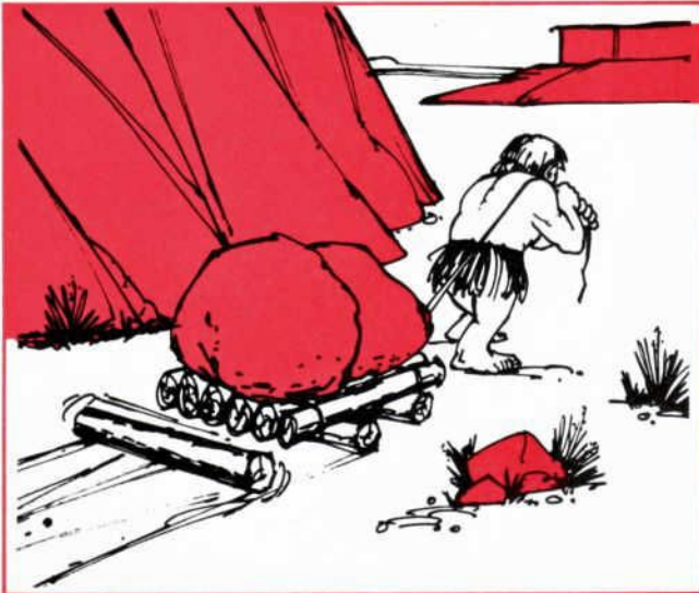
Figure 4 — Placing a roller under the load makes the job easier.
