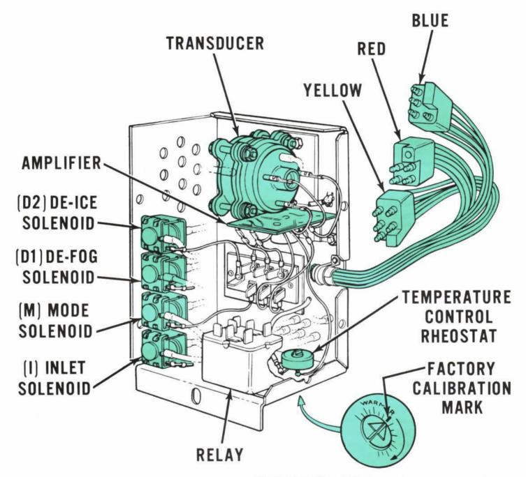
TEMPERATURE CALIBRATION ADJUSTMENT
