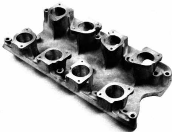
FIGURE 40. Falconer-Dunn manifold for Weber carburetion.
