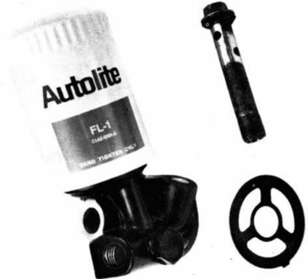
FIGURE 33. Oil cooler adaptor (C9ZZ 6881-A).
