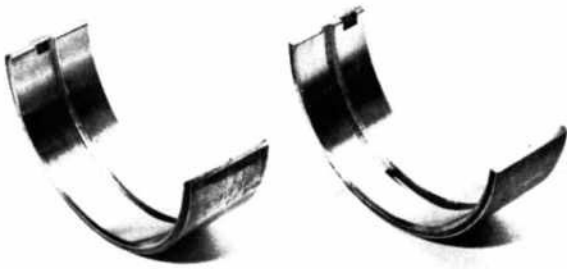
FIGURE 4. Fully grooved main bearing set.
