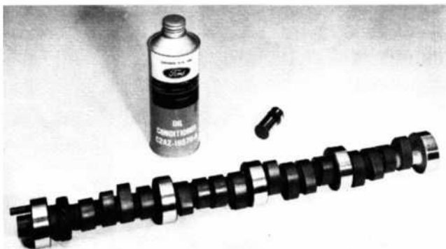
FIGURE 10. Cam, tappet and oil conditioner from competition only camshaft kit (DOZX 6250-B).
