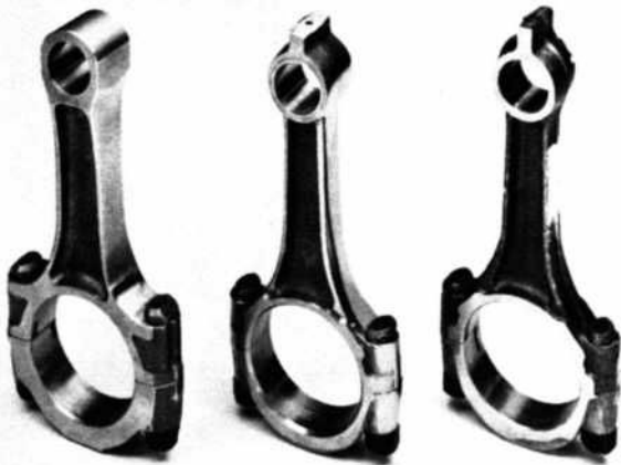
FIGURE 5. Boss 302 rods with stock rod on right. Center rod has been magnafluxed, polished and shot peened. Competition only rod ( DOZX 6200-A ) is on left.
