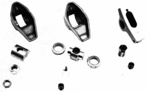
FIGURE 29. Boss 302 rocker arm assemblies showing stock on left, Ford competition setup in center (DOZX 6A585-A), and aluminum roller-type (non-Ford part) on right.
