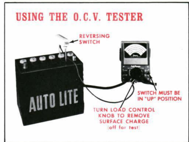
Figure 16—Using the O.C.V. Tester
