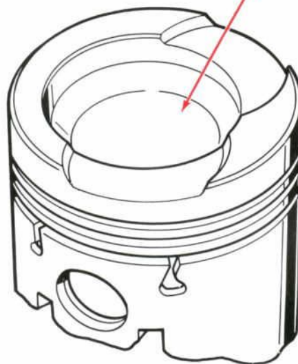
Figure 3—Cortina "Bowl-in-Piston" Design
