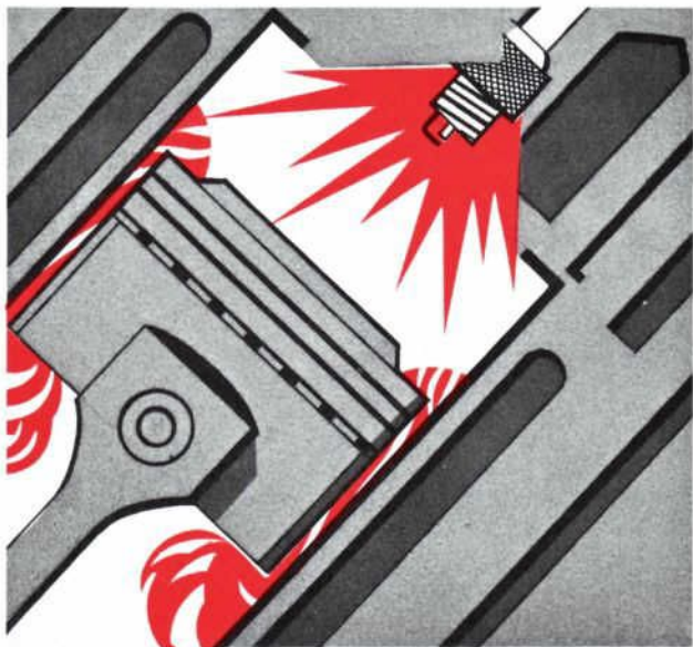
Figure 1—Combustion Produces Horsepower and Undesirable By-Products
