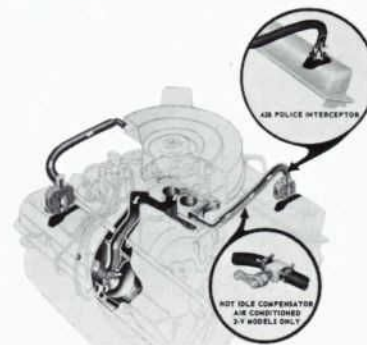
Figure 8—Aluminum Pack Oil Separator for 1968 390 and 428 Engines (Except 390 GT and 428 Police Interceptor)
