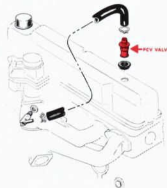
Figure 9—PCV Valve Location—6 Cylinder Engines
