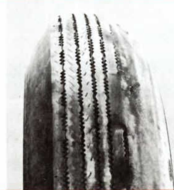
Figure 5—Too much wheel camber caused this uneven tire wear condition
