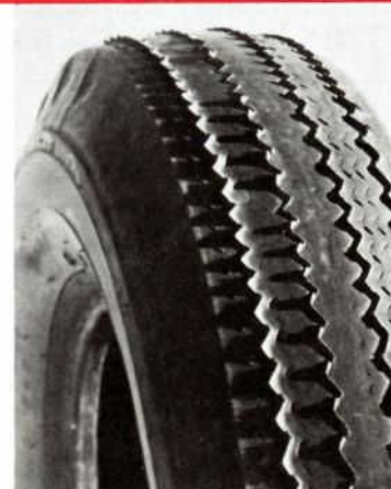
Figure 6—Misalignment of the wheels caused the feathered edge on the tread of this tire
