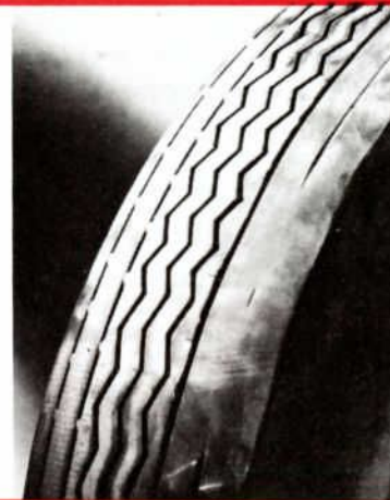
Figure 4—A single spot or series of cuppings around the tire circumference caused by a combination of underinflation and mechanical irregularities
