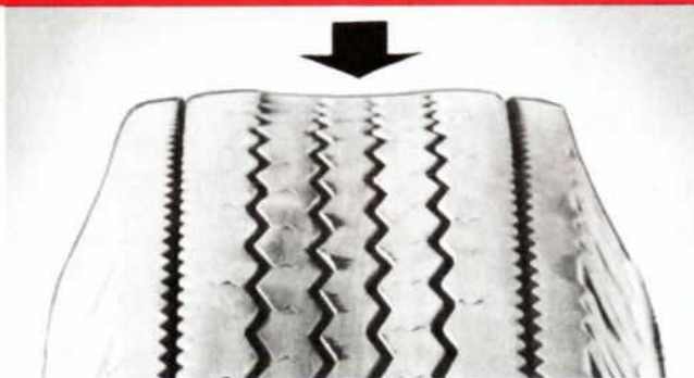
Figure 2—Abnormal tire wear caused by overinflation
