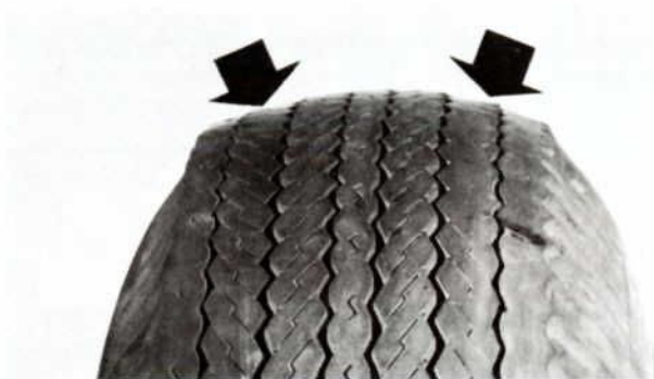
Figure 1—Abnormal tire wear caused by underinflation
