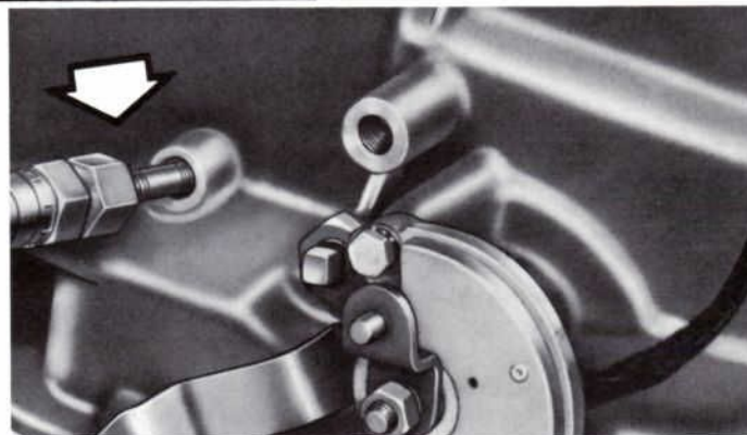
Figure 4—Control Pressure Gauge Connection
