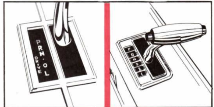
Figure 2—C6 Transmission Selectors: Automatic (L) Fairlane Sports-Shift (R)
