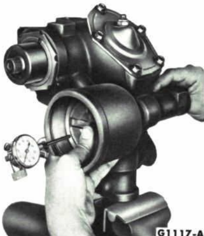
FIG. 44—Piston Backlash Check
