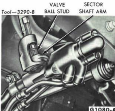
FIG. 29—Control Valve Ball Stud Removal
