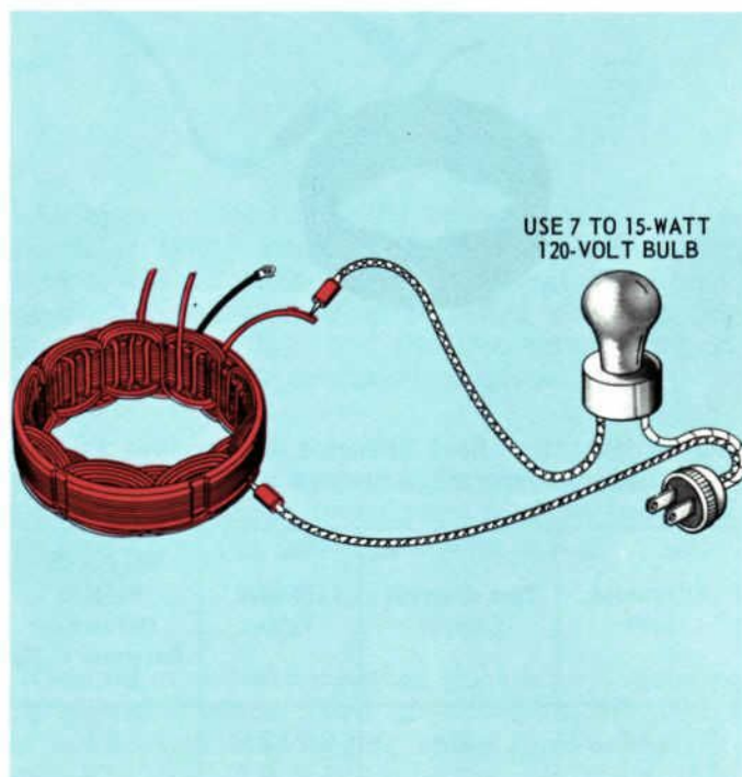
Fig. 31—Testing Stator Ground
