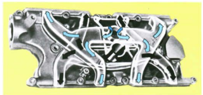
FIGURE 31. INTAKE MANIFOLD AIR-FUEL DISTRIBUTION PATTERN
