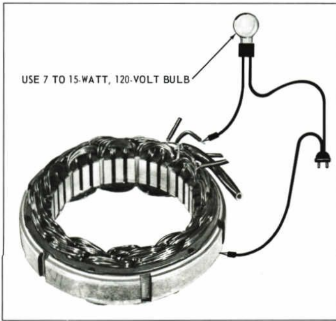
FIGURE 35. STATOR WINDING GROUND TEST
