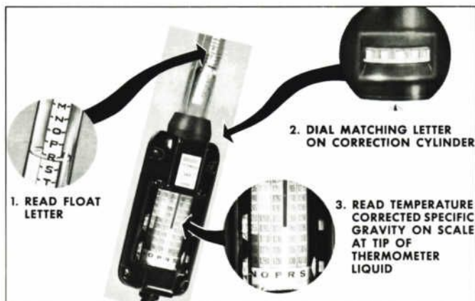
FIGURE 22. BATTERY HYDROMETER TEST
