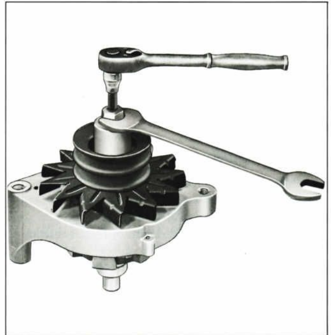
FIGURE 55. ALTERNATOR DRIVE PULLEY REMOVAL
