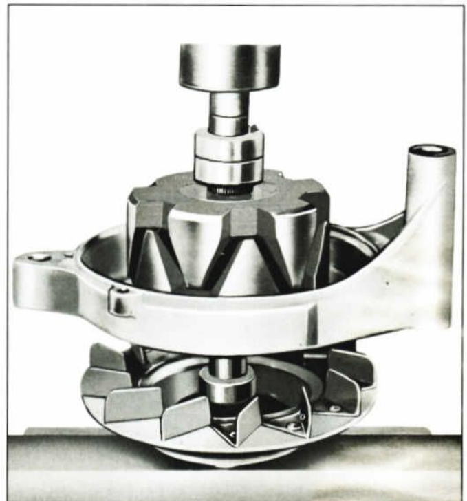
FIGURE 51. INSTALLING ALTERNATOR PULLEY
