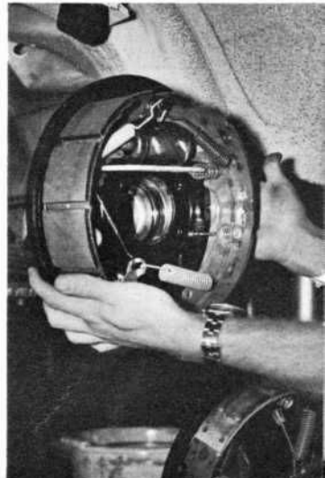
CONTROL ARMS are added to rear, extend forward into car body. Wider, segmented brakes are substituted for stock units.
