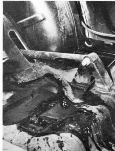
CONTROL ARMS are added to rear, extend forward into car body. Wider, segmented brakes are substituted for stock units.
