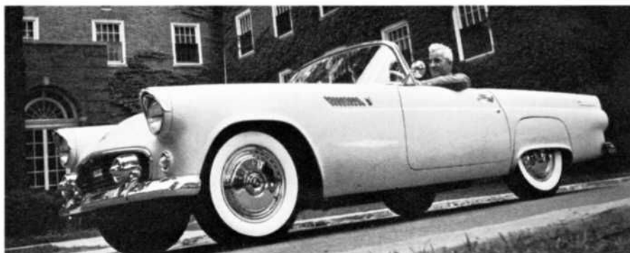
FIRST THUNDERBIRD was the 1955 model, of which 15,286 were sold. It featured "sporty" car concept with good-performing 292 cu. in. V-8 on 102-in. wheelbase.
