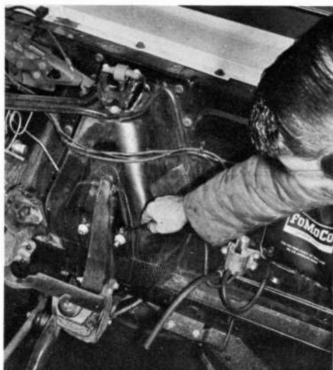
FRONT DISCS are standard Mustang items; upper arm mounting points are lowered; rear axle is fitted with Konis.
