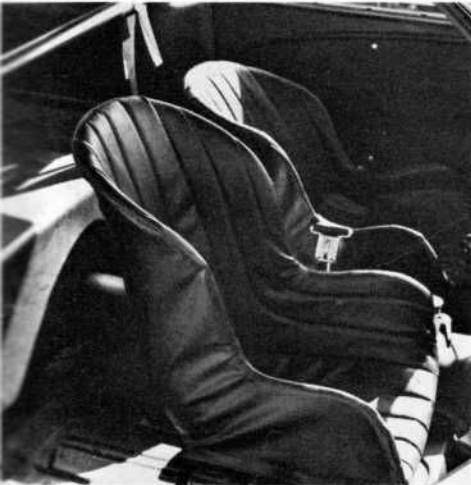
COMPETITION VERSION is much more stark; real bucket seats replace Detroit types; hefty roll bar is optional, but fully-instrumented dash is part of the race-ready package. All frills are removed.
