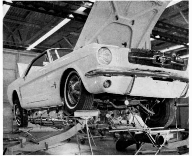
STRAIN GAUGE indicators measure torsional rigidity during bending tests in the Ford Engineering Center's structures lab.
