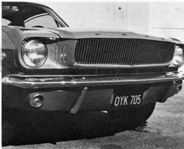
VERTICALLY-BARRED "Elegant" grille from Products d'Elegance is an easy, 20-min. swap for the standard Mustang trim.
