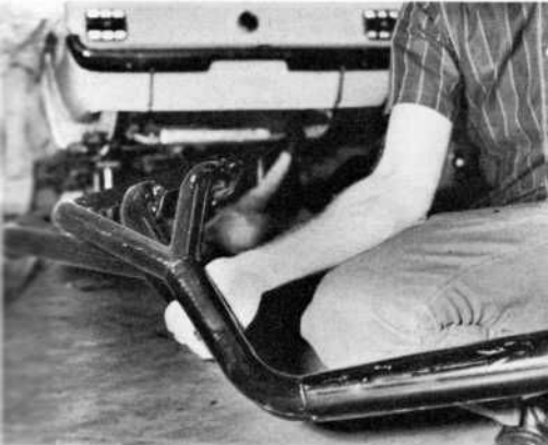
HUGE HEADERS are used with the racing-prepared engines. Hole in hood matches up with air horn atop the carburetor to give pressurized flow of cool air. Street engines have stock air cleaner; racing engines, air horns.
