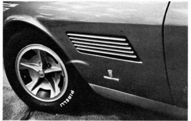
ITALIAN-STYLED "mag-type" wheels are cast in a magnesium alloy. Pirelli Cinturato tires, 195-14, are mounted on the 6L x 14 rims.
