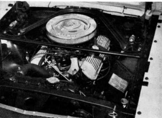
NORMAL GT-350 engine has horsepower increased by bolt-on treatment, such as the high-riser intake manifold. Valve covers are for show. Competition oil pan, however, has added capacity for better cooling.
