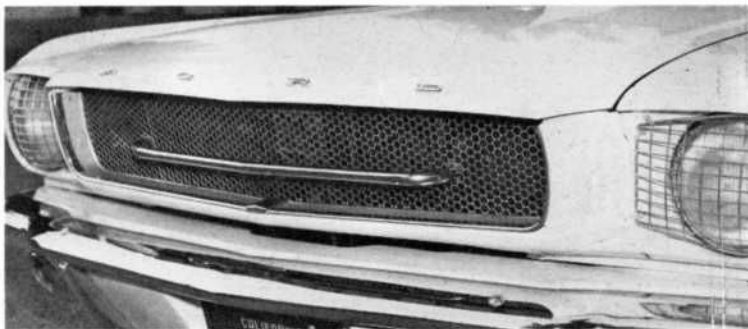
HEADLIGHT COVERS of plastic from Weiler; right, EELCO's gas cap. GRILLE BAR and bull nose pieces from EELCO.
