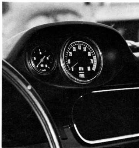
INTERIOR TREATMENT of "street" GT-350 includes 3-in. wide safety belts, wood-rimmed steering wheel, electric tachometer and oil pressure gauge in pod atop dash, and back seat replaced by fiberglass cover.
