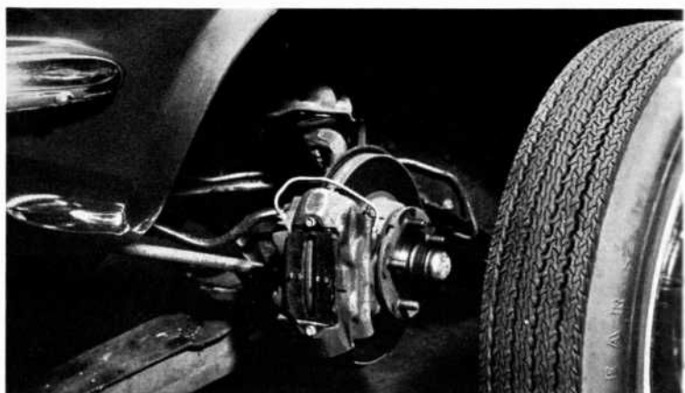
DISC BRAKE used on Mustang consists of ventilated, 11.375-in. disc and 4-cyl. caliper. Pads are easily exchanged for new.
