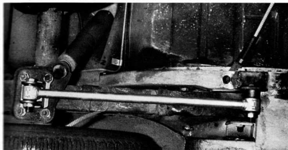
TRACTION MASTER arms mount beneath leaf springs and provide improved rear axle control. Forward bracket must be welded in place.
