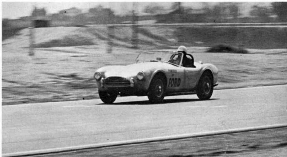
EARLY TRACK tests at Riverside Raceway revealed some amazing performance characteristics; 0-100 in 10.8 sec., top speed over 150 mph, fine handling.
