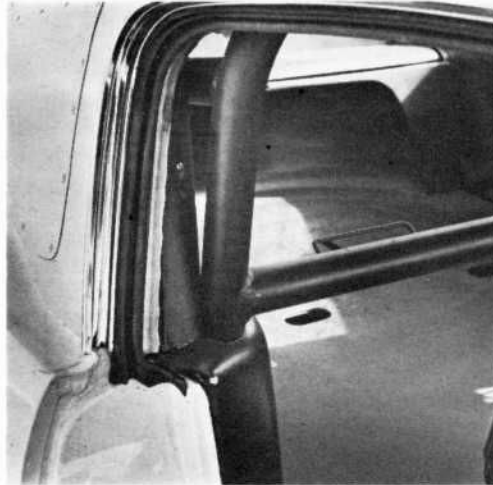
COMPETITION VERSION is much more stark; real bucket seats replace Detroit types; hefty roll bar is optional, but fully-instrumented dash is part of the race-ready package. All frills are removed.
