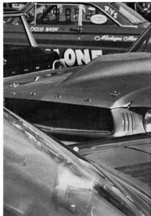
HOOD scoops on the A/FX cars have vents in back to let in cool air for carburetors. Oil pressure gauge shows through screen.
