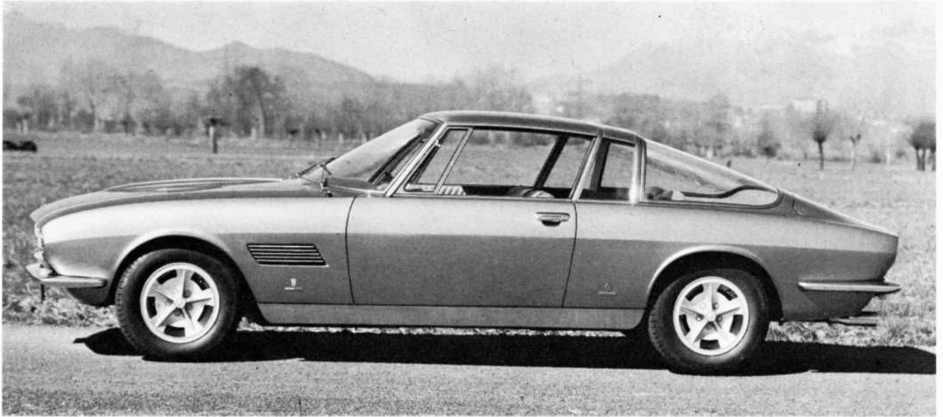
ITALIAN-STYLED "mag-type" wheels are cast in a magnesium alloy. Pirelli Cinturato tires, 195-14, are mounted on the 6L x 14 rims.
