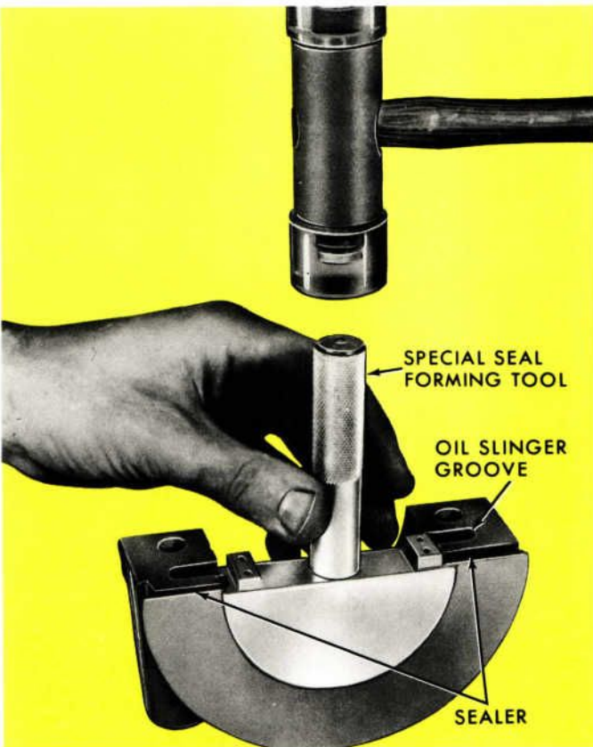
FIGURE A-7. SEAL-TO-REAR MAIN BEARING CAP INSTALLATION
