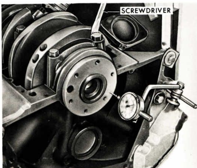
FIGURE A-8. CHECKING CRANKSHAFT END PLAY
