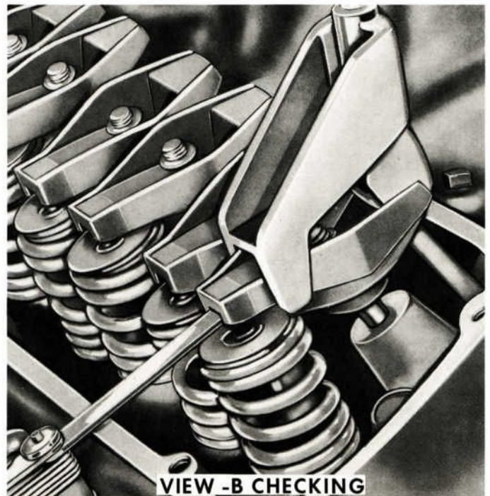
FIGURE A-19. ADJUSTING AND CHECKING VALVE CLEARANCE
