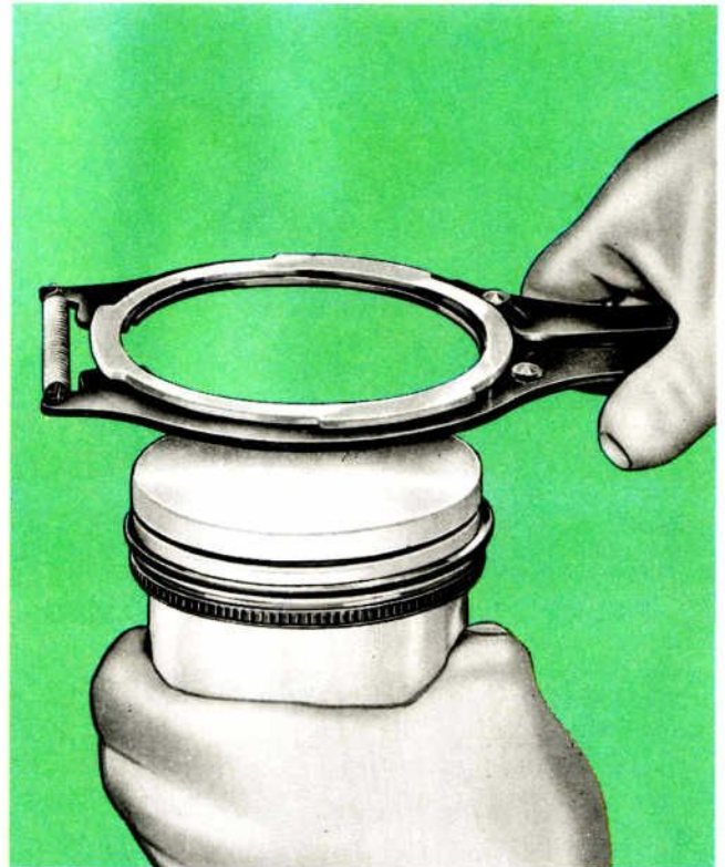
FIGURE A-13. INSTALLING PISTON RINGS
