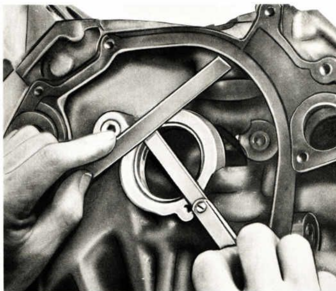
FIGURE A-2. MEASURING FRONT CAM BEARING DEPTH
