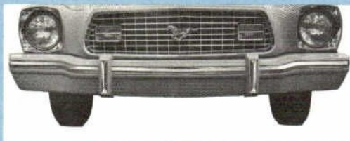
The Mustang Look —One-piece front end with integrally styled urethane covered bumper
