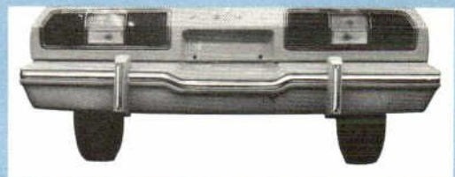
Touch of European Styling —Traditional Mustang three-pod taillights with center amber turn signal
