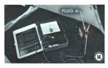
If the ohmmeter reading is less than 4 ohms, inspect the solenoid wires for a ground to the floor pan or other body surfaces. Repair or replace any solenoid wires that are grounded and perform a functional test.
