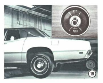
4. Move the transmission selector lever to the "D" drive position, with the engine at normal operating temperature; accelerate to approximately 25-30 miles-per-hour on the speedometer, with both rear wheels turning. CAUTION: Never exceed 60 miles-per-hour on the speedometer to avoid possible damage to the car. If both rear wheels do not turn, correct any difficulty, such as brakes too tight or rear axle damage, before continuing the functional check.
