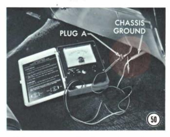
If the ohmmeter reading is one ohm or less, the system has a good ground. Therefore, the problem is in the control module; replace the control module and perform a functional check.
