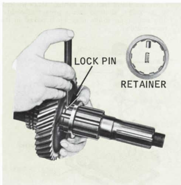
Removing Second-Speed Gear Thrust Washer — New Process 541 Five-Speed Transmission
