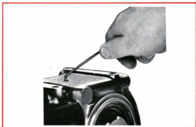
Figure 9—Making an Oil Level Check at the Compressor
