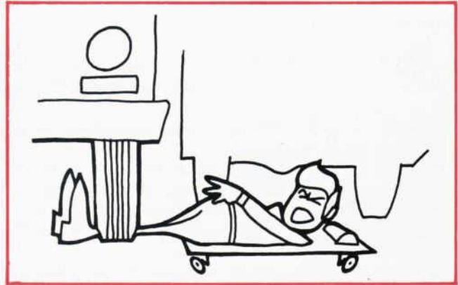
Figure 16—Arms and legs sticking out from under a car can lead to serious injury. Drivers of other cars pulling into the adjacent area may not be able to see you. Protect yourself and avoid injury.
