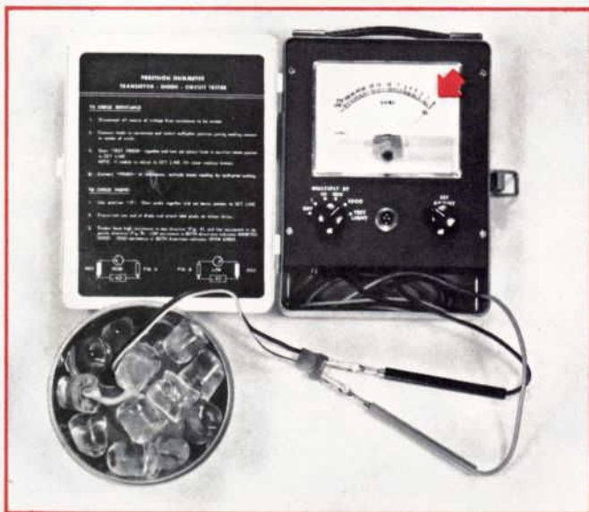
Figure 22—Testing the Thermal Switch to See if it Closes When Chilled
