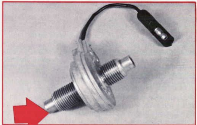
Figure 5—The Speed Sensor and Sintered Bronze Bushing
