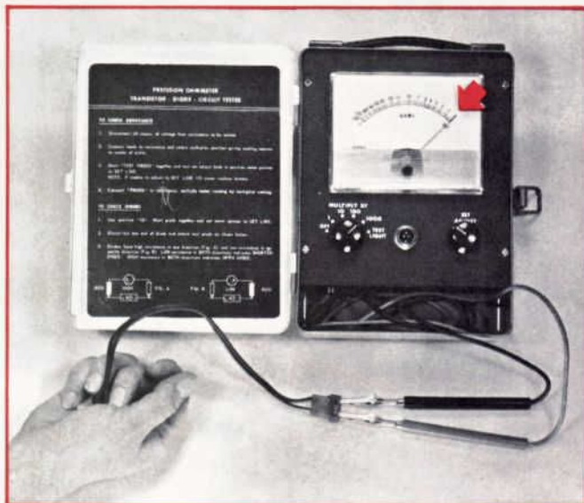
Figure 21—Testing the Thermal Switch with an Ohmmeter. No Reading Means the Switch is OK
