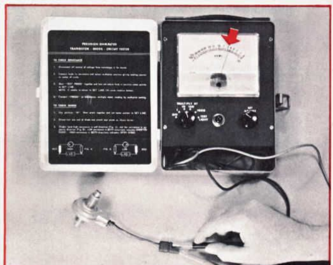
Figure 27—Checking Speed Sensor Continuity Using an Ohmmeter
