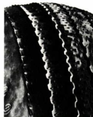
Figure 5—Feathering Due To Misalignment or Severe Cornering
