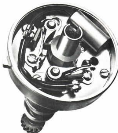
Figure 4—New Dual-Point, Dual-Advance Distributor
