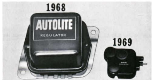
New and Old Voltage Regulators
