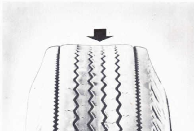
Figure 8— Overinflation Wear occurs at the center of the tread area. Causes early failure in the center of the ribs or sidewall areas.
