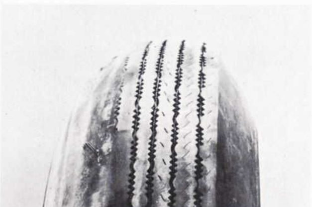
Figure 6— Camber Wear resulting from out-of-spec camber adjustment, produces excessive wear on the inner or outer shoulder of the tire, usually one side only.
