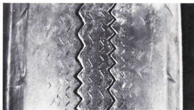
Figure 7— Cornering Wear also produces excessive wear on the inner and outer shoulder of the tire due to fast driving on curves and around corners, usually on both inner and outer shoulders.
