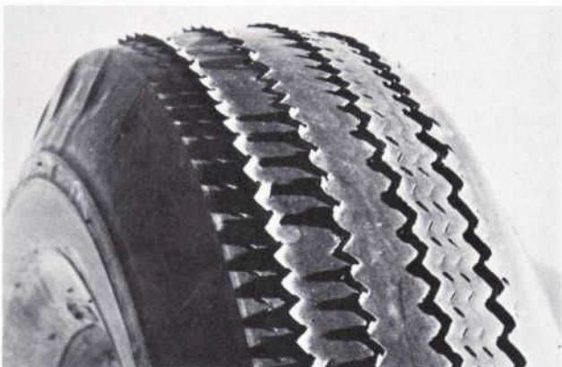
Figure 5— Toe-in or Toe-out Wear produces a feather-like edge along the edges of the tread due to a scrubbing action on the road. Excessive Toe-in produces a feather edge on the inner edge of the tread. Toe-out produces a feather edge on the outer tread edge.
