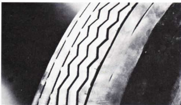
Figure 4— Spotty Wear occurs along the edge of the tire in small circular areas. It's caused by a combination of conditions, including tread design, inflation pressure and misalignment.
