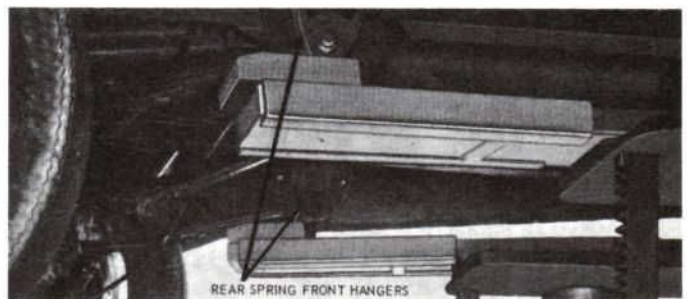
Figure 4—Rear Hoist Adapter Pad Position
