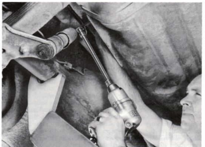
4. On Station Wagons only, use an impact wrench with an extension and, holding the upper bolt with a box wrench, remove the upper nut.
