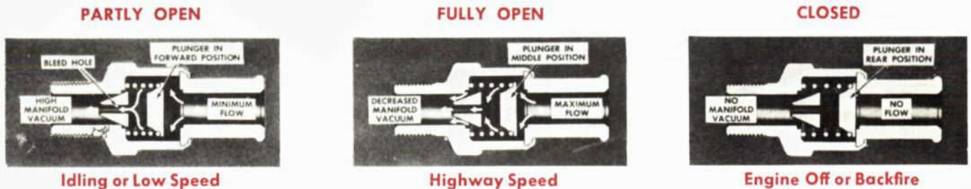
Figure 2—Emission System Valve Operation
