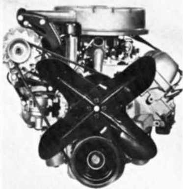
Latest thin-wall casting techniques are used in the manufacture of the 330-cubic-inch Oldsmobile block for lighter weight and better casting.
