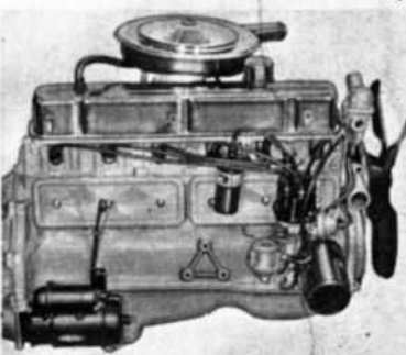
1. First engine is 153-cubic-inch power-plant offered as companion to larger six-cylinder in the Chevy II and Chevelle. Second engine is the 194-cubic-inch six-cylinder, while last engine is 230 six.
