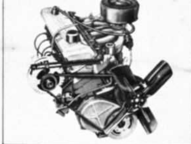
1. The Chrysler slant six engine, with positive crankcase ventilation.
