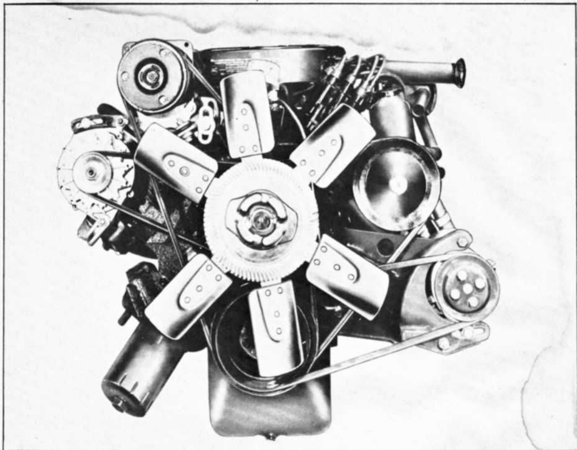
Above: This shows the thermostatically controlled fan, and the many accessories driven by the front pulley. Clockwise, from left, are the alternator, air conditioner, power steering pump, and exhaust emission control pump.
