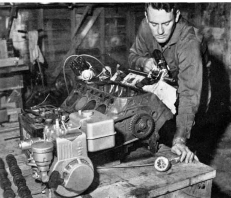
Karol devised his own camshaft and valve gear test machine using an old Y-V8 block, one head, train for two valves, a stock distributor and timing light. Small utility engine turned camshaft to desired rpm, timing light stopped action.
