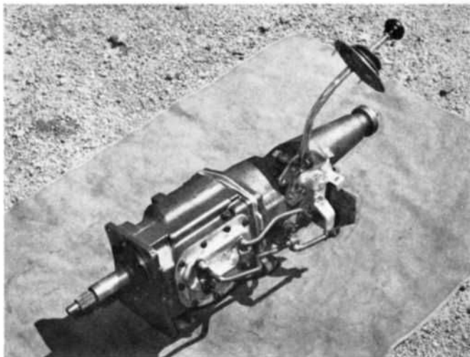
This is Ford's 4-speed transmission in cast iron with aluminum side cover, by Borg-Warner company. It comes with ratios of 2:37, 1:78, 1:37 and 1 to 1. Shift lever has reverse lock out.
