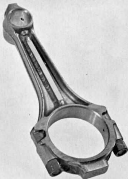
LEFT —406 rods are very strong but Crankshaft Co. adds a rib on either side for use in stroker kits or with blowers. CENTER —Aluminum rods are also popular among rodders. This one by Howard is made with forging process for high strength. RIGHT —Jahns Piston Co. makes any style desired for Ford. Top, domed 12:1 piston for 390 Ford; bottom, 10.5:1 Falcon.
