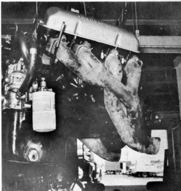
Late cast iron headers for the 406 engine are tuned to exhaust impulses, have large capacity branches. On left side, 1st and 3rd cylinders hook together, 2nd and 4th together. On right side of engine 1 and 2 are together, and 3 and 4 are together.
