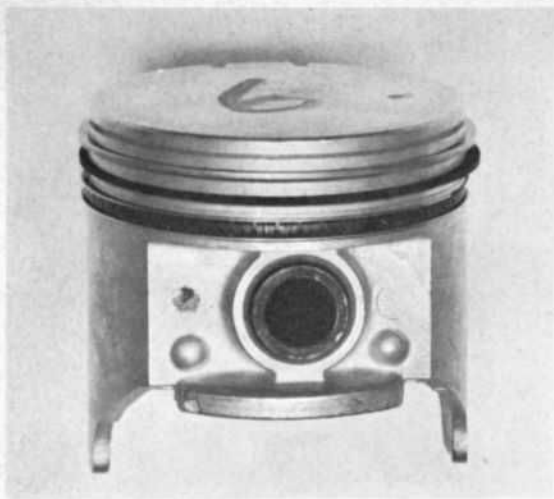
Fairlane V8 piston is cast aluminum, slipper skirt design. Top groove acts as heat dam to protect rings.
