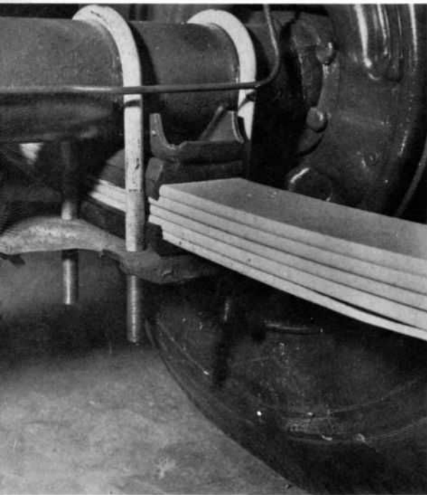
Standard U-bolts have shoulders which will prevent overtightening. Service bolts shown have no shoulder, can be tightened to compress rubber insulators.
