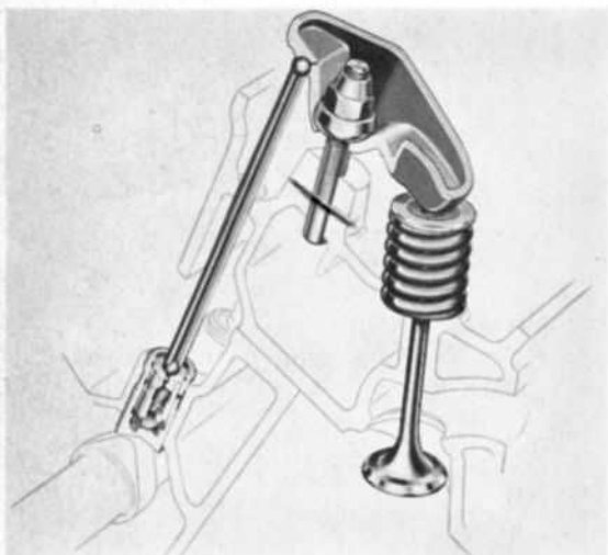
Valve train layout is shown for 221-.60 V8. Pushrod tubes have ball bearing ends. Rocker studs press into head. The rocker pivot ball is sintered metal.
