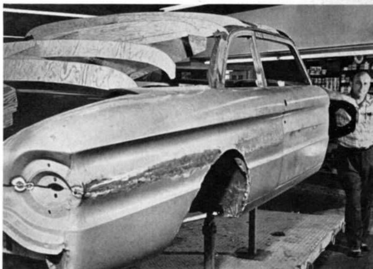
Holman stands beside unfinished "Challenger III," a Falcon which is being chopped six in. and fitted with bored-out, 221-in. Fairlane engine which makes it eligible for G.T. road racing.
