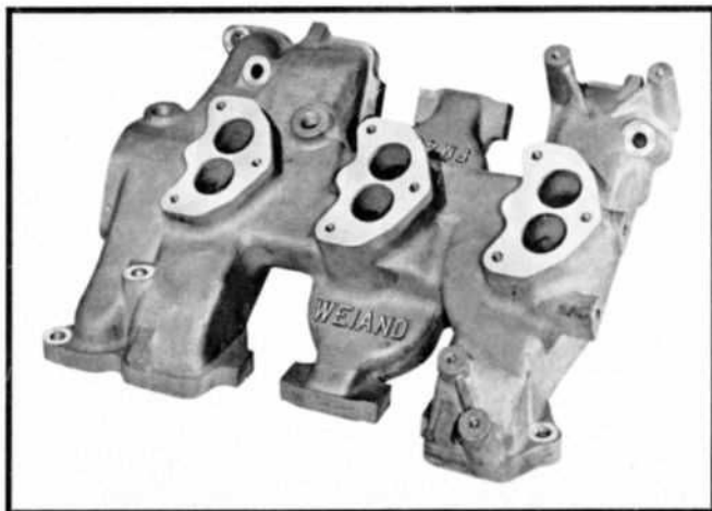
Weiland three-carburetor intake manifold for Y-V8 Ford and Merc 272-312 engines has exhaust heat to the bottom of the passages to improve fuel vaporization, give smooth operation.
