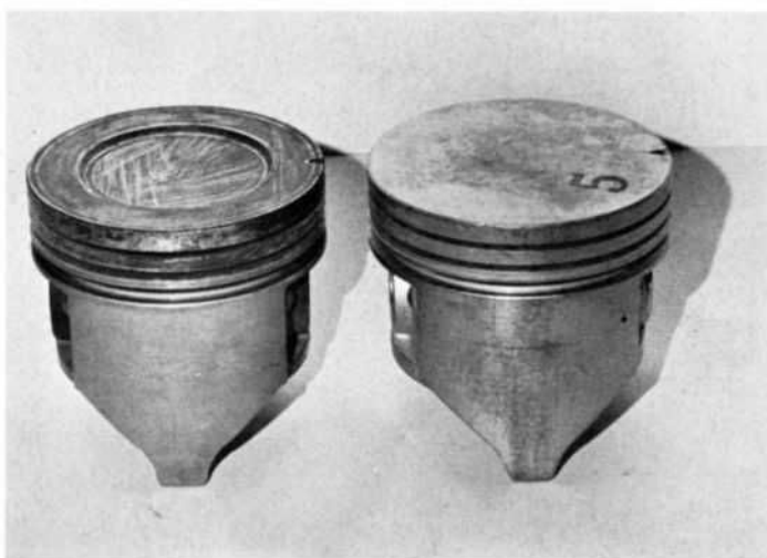
LEFT—Connecting rods for the 406-inch high performance V8 (left) are much stronger, slightly heavier than those used in standard engines (right). ABOVE—Pistons for high performance 390 engine (left) have recessed top. 406 pistons have flat top but there is more clearance between the piston and block deck.
