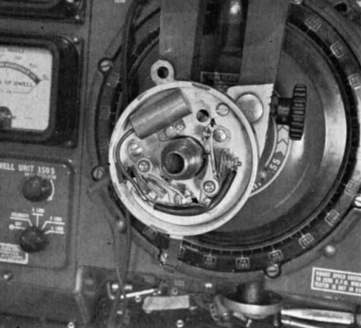
Left: A distributor Strobe is essential if exactness is to be accomplished. This is the only way to set the cam angle electrically, set proper advance rate, and check point bounce and condenser performance. Right: Centrifugal advance mechanism only is used on Ford high performance 352 to 406 engines. Return springs and weight action should be checked carefully on the distributor machine to make absolutely certain that the action is smooth and that the proper advance curve has been obtained.
