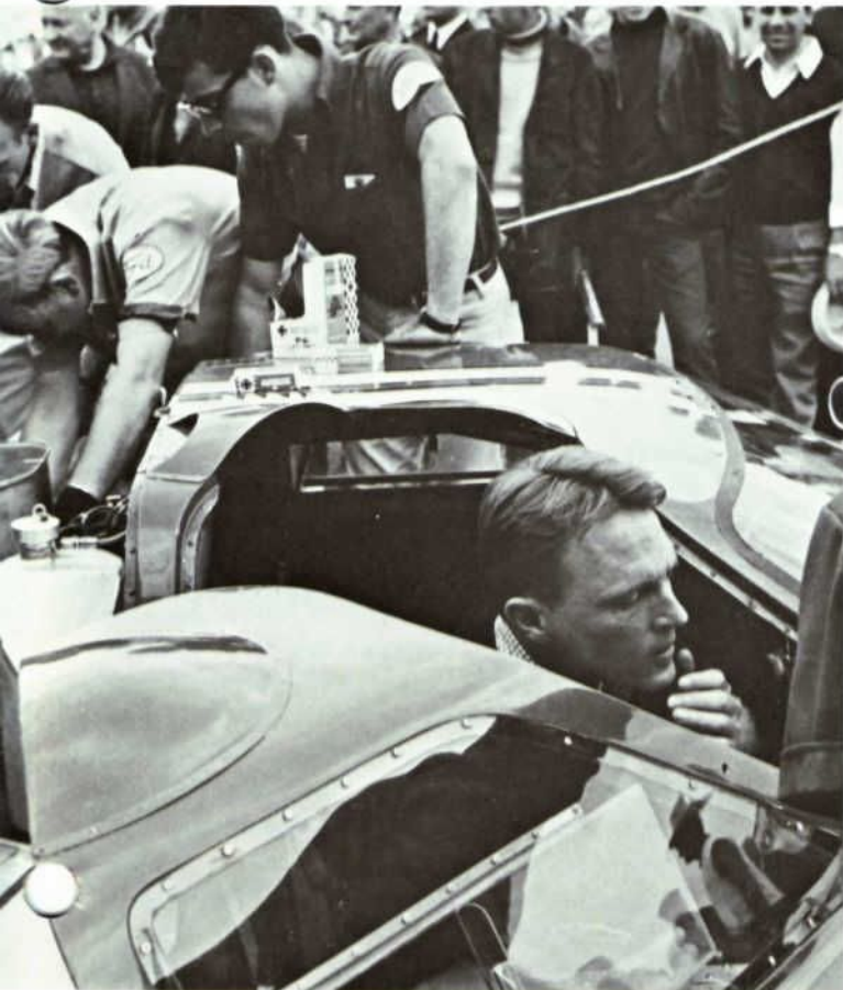
A small bubble was added to the roof to provide more headroom
