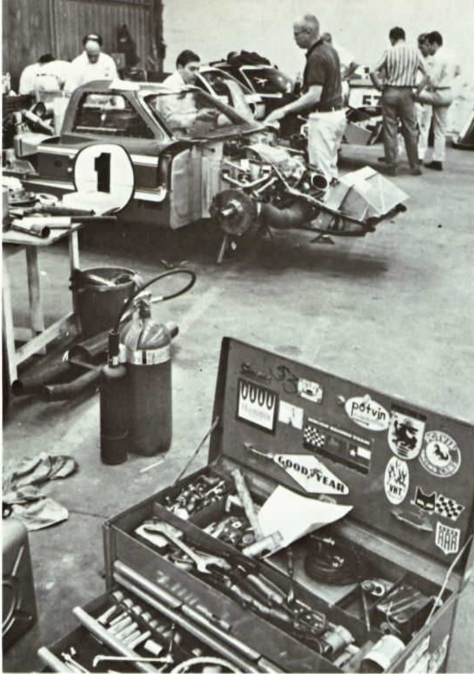
The Mk. IV, like the other Ford teams, was powered by a seven-liter, or 427-cubic-inch Ford engine, which pulled about 500 hp
