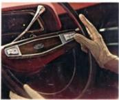
Automatic Speed Control (Ford, Thunderbird), a better idea for freeway driving. Preset speed. Cruise with foot off accelerator. Mustang version is called Fingertip Speed Control.
